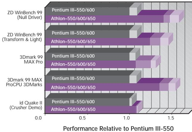
Figure 8. 3D benchmarks indicate Athlon's 3DNow implementation is a match for P III's SSE. (Source: AMD)
