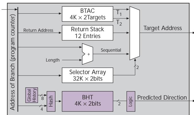
Figure 5. Athlon uses the Gshare variation of a two-level branch predictor to predict branch direction. Target addresses are predicted by a BTAC integrated into the instruction cache.
