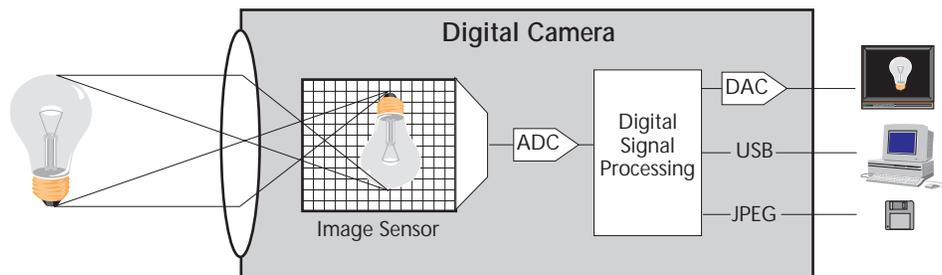
Figure 1. In a digital camera, the image is focused on an image sensor made up of an array of light-sensitive elements (pixels). Analog signals corresponding to the intensity of light falling on each pixel are converted to digital values by the ADC and processed into a final color image by digital-signal-processing circuits.
