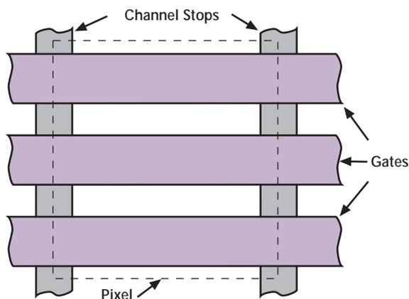
Figure 2. In a CCD, photons striking the pixel are converted to charge by the photoelectric effect and stored in the depletion-region beneath the gates formed by the gate potentials. These charges can be transferred from pixel to pixel down the array by modulating the gate voltages with carefully timed clock pulses. Channel stops isolate pixels in one column from those in the next.
