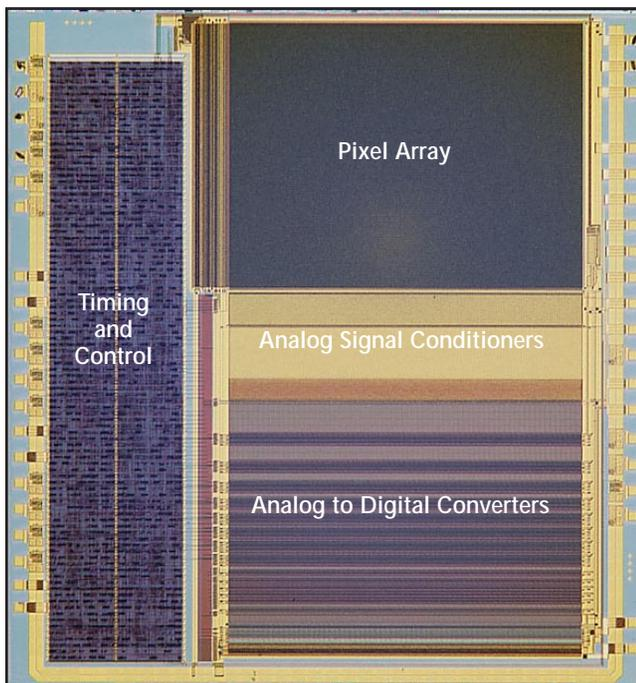
Figure 4. Photobit's PB159 CMOS image sensor is  $8.6 \times 9.4$  mm with 196,608 ( $512 \times 384$ ) active pixels and column-parallel analog-to-digital converters. Each pixel is  $7.9 \times 7.9$  microns.
