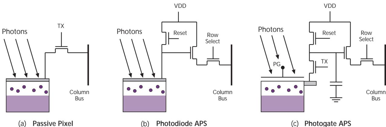
Figure 3. Early CMOS image sensors used a passive-pixel arrangement. But CMOS scaling now allows active pixels, which have amplifiers at each pixel site to improve the light sensitivity and signal-to-noise ratio.
