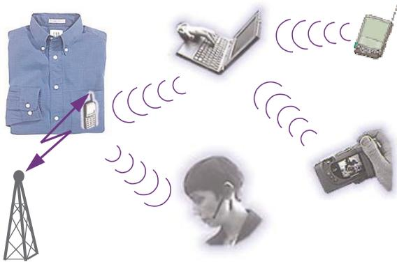
Figure 1. No more cables! Bluetooth uses an RF link to connect all your personal devices, such as notebook computers, PDAs, cell-phones, headsets, and digital cameras.
