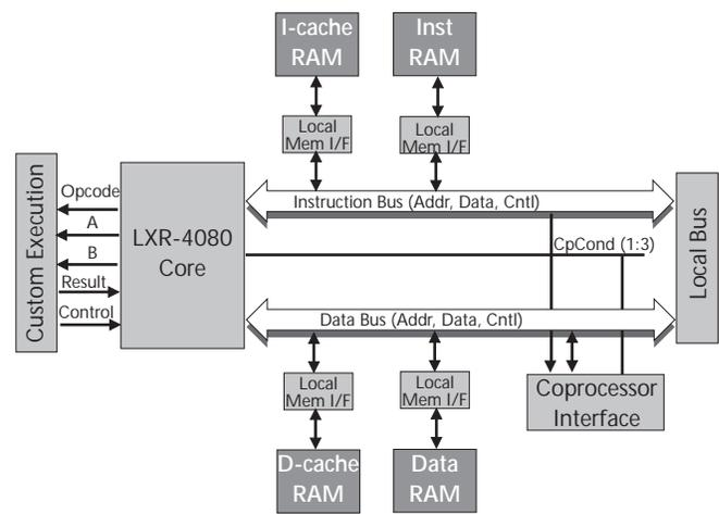
Figure 1. Lexra's LXR-4080 MIPS core includes, at a minimum, the CPU, two caches, and an internal bus interface. The CPU core can be extended either with coprocessors or with custom logic.
