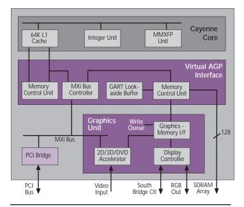
**Figure 1.** The Cyrix MXi includes the general-purpose Cayenne core for x86 compatibility and enhanced 3D-geometry performance, an AGP-compliant memory controller and graphics interface, and an integrated 2D/3D/DVD graphics subsystem that should match or beat the performance of discrete solutions.
