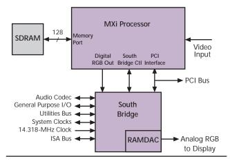
Figure 2. The MXi processor comes with its own "south bridge" chip that includes a RAMDAC and ISA bridge. OEMs can produce complete systems by adding a few commodity peripheral chips.
