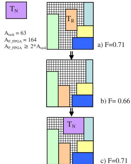
Figure 6. FPGA status before (a) and after (b, then c) an on-demand defragmentation.
