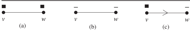
Figure 1. Orientation helps in symmetry breaking. In Figure (a) both v and w choose the same color. In (b), for existing algorithms both remain uncolored whereas in (c), when using orientation, node v may get colored.
