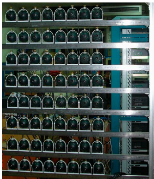
Fig.2. A photo of our 64-camera light field camera array. The cameras are arranged in rows of eight.
