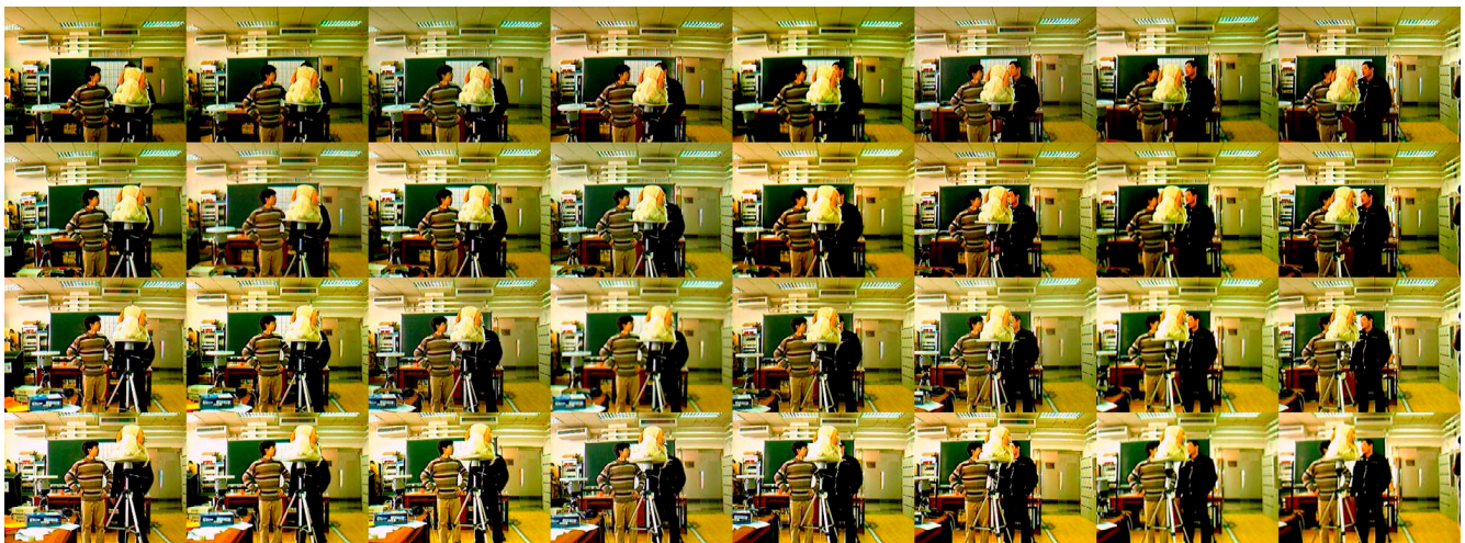
Fig.5. Half of views in the first field of DLF sequence taken with our light field camera
