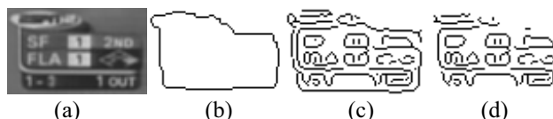
Fig. 3. The results of the contour and layout extraction process; (a) a caption region; (b) a contour image; (c) an edge image; (d) the layout of the caption image.
