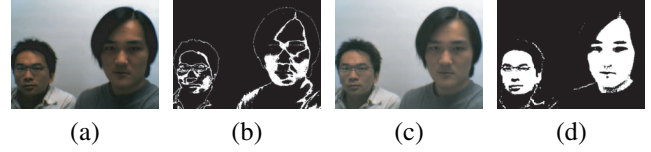
Fig. 3. An example of dark image compensation: (a) original dark image (b) the S_{ij} without compensation (c) compensated image (d) the S_{ij} of compensated image.
