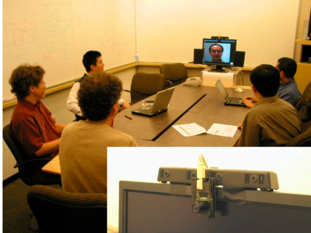
Figure 1. The meeting room; the PING stand-in device is at the end of the table, and consists of a flat panel monitor, a linear microphone array, a wide-angle camera, and two loudspeakers.
