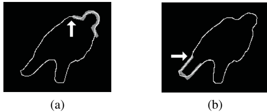
Fig. 6. Best fitting positions of templates for a human silhouette represented by a snake; (a) head, (b) limb (leg).
