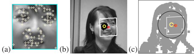
Fig. 3. (a)sparse template, (b)template during tracking (white frame); black cloud : particle distribution, larger circle : center point of template (head center), smaller circle : center of template surface. (c)extracted foreground region (gray area) and estimated head circumference (circle).
