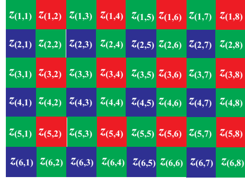
Fig. 3. Bayer CFA with the GRGR phase in the first row [5].
