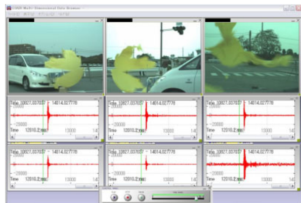
Figure 7: Results of synchronous recording of video and sound in collision scenario.
