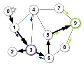
**Figure 2.** Semi-probabilistic routing with  $\phi=1$  and  $\tau=0.5$ . Numbered circles represent dispatchers. A colored circle around a dispatcher denotes it as a subscriber. The short colored arrows represent subscription information, and indicate the forwarding path for matching events. Dispatcher 0 publishes an event that gets forwarded either deterministically (double-headed thick arrows) or probabilistically (single-headed thick arrows).
