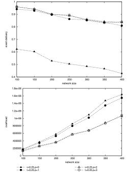
**Figure 7.** Event delivery and overhead in a dynamic network with reconfigurations every  $\rho = 0.03s$ .
