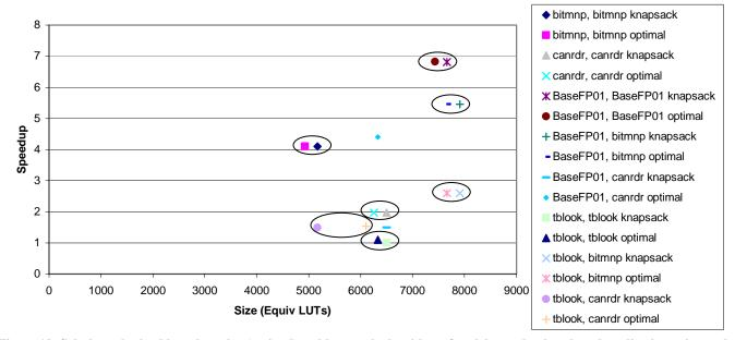
Figure 10: Solutions obtained by exhaustive (optimal) and knapsack algorithms, for eight randomly-selected application pairs, and an area constraint set to 80% of the area of the best configuration. The knapsack algorithm finds near-optimal solutions for seven of the eight pairs (circled), doing poorly on one pair (the two non-circled points).
