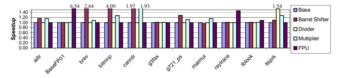
Figure 6: Speedups for each instantiatable unit, for each benchmark. Instantiating particular units can have significant speedup impacts.
