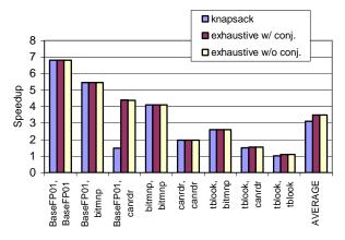
Figure 11: Speedup of the chosen benchmark pairs, using the 80% of the best configuration size constraint.
