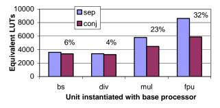
Figure 3: Sizes of two-processor systems with two separate units (sep), or one conjoined unit (conj). % size savings from conjoining are shown, showing significant savings.
