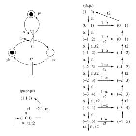
Figure 3: A TGMG and its Markov chain for the bounded  $(\delta(t_1) = \delta(t_2) = 1)$  and unbounded case  $(\delta(t_1) = 1, \delta(t_2) = 2)$ .
