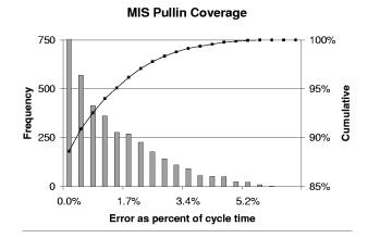
Figure 4: Graph of min-delay (pullin) errors.
