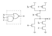
Figure 2: Static Gate  $o = \overline{(a + bc)}$
