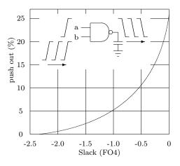
Figure 1: MIS Maximum Delay Pushout Effect
