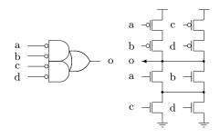
Figure 5: Gate  $f = \overline{ac + ad + bc + bd}$
