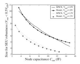
Figure 2: This figure illustrates the accuracy of the compact robustness model given by Eqn. (10) for a 2-input nand gate for a dual- $V_{\rm DD}$  technology. It is clear that the optimum size for SEU robustness is estimated to within 0.5 times the size of the unit-scaled gate over the range of circuit configurations.
