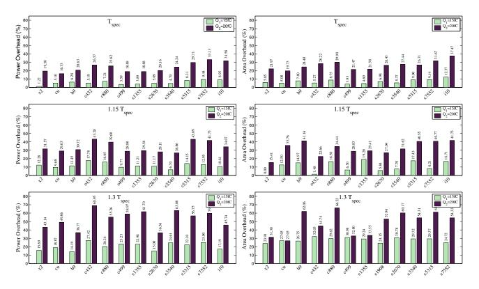
Figure 4: This figure presents power and area overhead (in %) when the benchmarks are optimized to meet a delay constraint of  $T_{\text{spec}}$ ,  $1.15 T_{\text{spec}}$ , and  $1.3 T_{\text{spec}}$  on all outputs using simultaneous dual- $V_{\text{DD}}$  and gate sizing. The power and area overhead required for SEU robustness increases from high performance ( $\Delta = T_{\text{spec}}$ ) to low performance ( $\Delta = 1.3 T_{\text{spec}}$ ) designs (explained in Sec. 4.3).
