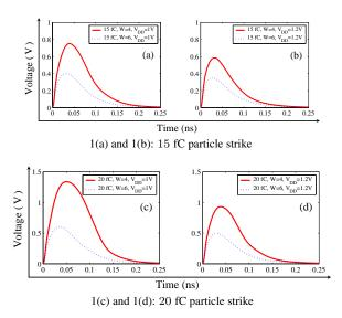
Figure 1: SPICE simulations of particle strikes of 15 fC and 20 fC charge at a nand gate, whose size and  $V_{\rm DD}$  are varied.
