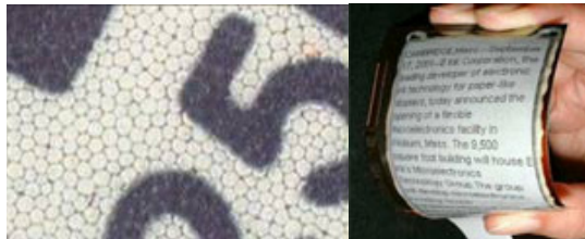
Figure 2. Capsules containing colloidal suspension in an EPD display (Flexible Display Center, ASU, E-Ink Corp.)
