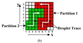
Figure 4: (a) Detectors used in bioassay; (b) Routing result and array partitions.
