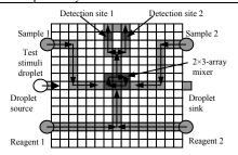
Figure 12: A 15×15 array used for multiplexed bioassays.
