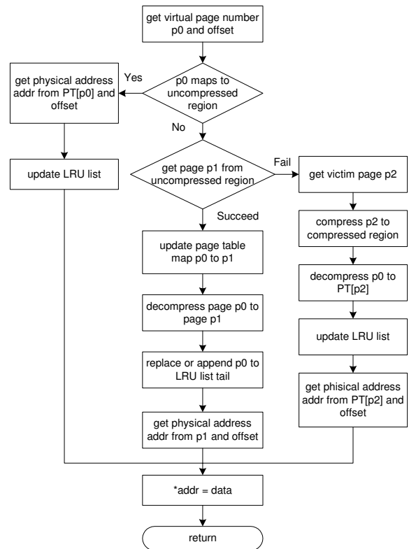
Figure 2: Write handle procedure
