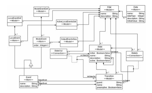
Figure 3: A Class Diagram for the FML Metamodel
