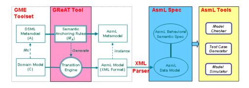
Figure 1: Experimental Tool Suite for Semantic Anchoring
