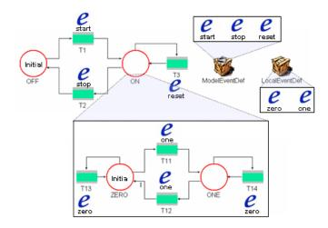
Figure 5: Hierarchical FSM Model for Checksum Machine
