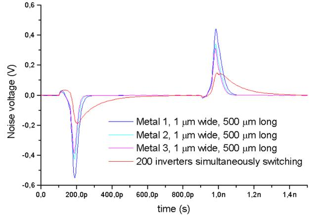
**Fig. 7 Noise waveforms originated by switching interconnects compared against those originated by 200 simultaneously switching CMOS inverters.**
