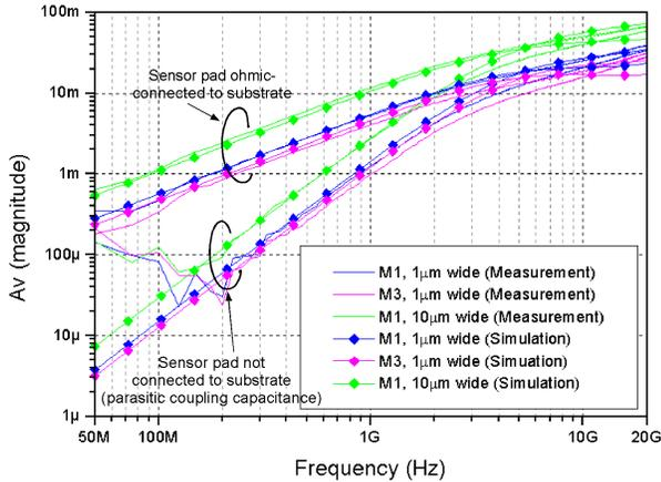
**Fig. 3 Voltage coupled from the interconnects to the sensor pads. Interconnect is open-ended.**
