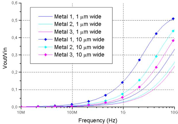
**Fig. 6. Noise levels coupled to substrate when a 1 V signal is applied to lines of different widths and metal layers.**
