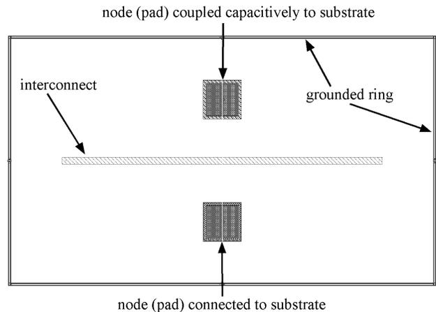
**Fig. 5. Layout of the basic test structure used in the simulations.**
