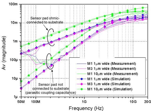
**Fig. 4 Voltage coupled from the interconnects to the sensor pads. Interconnect is 50 Ω loaded.**
