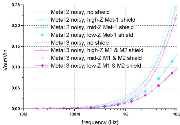
**Fig. 10. Noise levels coupled to substrate when a 1 V signal is applied to  $1\text{-}\mu\text{m}$  wide lines in metal-2 or metal-3. These lines are shielded by lower-layer metal lines, driven by high, medium or low impedances.**
