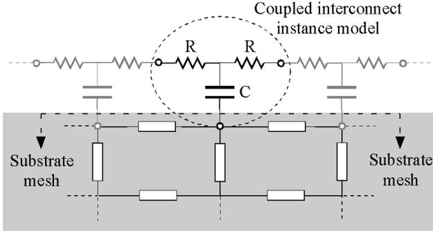
**Fig. 1. Equivalent circuit model for an interconnect coupled to substrate.**
