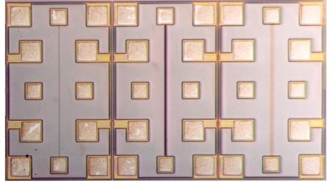
**Fig. 2. Test structures implemented in a 0.35  $\mu\text{m}$  technology to measure coupling from interconnects.**
