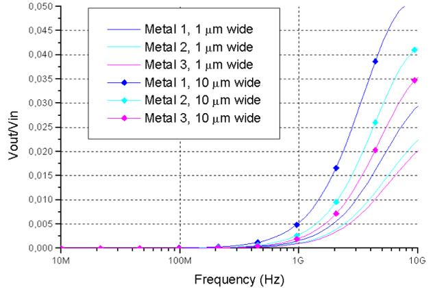
**Fig. 9. Noise coupled to a sensitive device through parasitic capacitance, when a 1 V signal is applied to lines of different widths and metal layers.**
