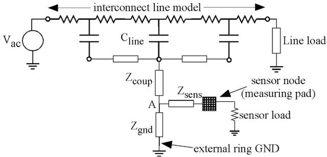
**Fig. 8. Simplified equivalent circuit for a noisy interconnect coupled through the substrate to a surface node (bottom half of structure in Fig. 5).**
