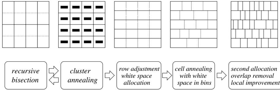
Figure 1: Our placement flow with two white space allocations.
