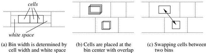
Figure 3: Simulated annealing after white space allocation.
