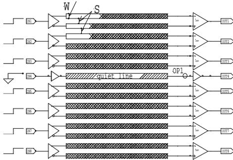
Figure 13: A 8-bit global bus with 7-bits differential (14 signal lines) 3000 $\mu$  long.  $W = 3\mu$ ,  $S = 1.5\mu$ . The non-differential (standard) bit signal is placed in the middle of the differential signals.
