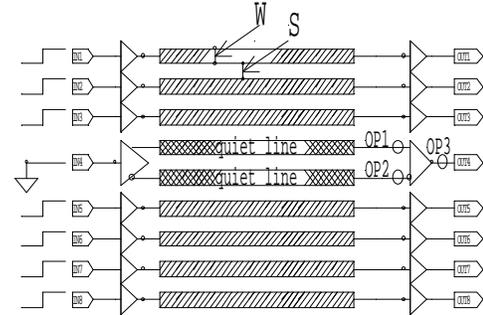
Figure 15: An 8-bit, 3000 $\mu$  long, global bus of 7 standard signals and a differential signal located in the center of the bus.  $W = 3\mu$ ,  $S = 1.5\mu$ . The bus is sandwiched between a VDD line and a VSS line. The driver of the differential signal is a limited swing differential driver and the receiver is a differential receiver. The drivers and receivers of all the standard bits are standard CMOS buffers.
