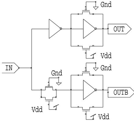
Figure 8: Limited Swing Differential Transmitter
