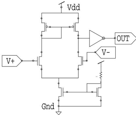
Figure 9: Differential Receiver
