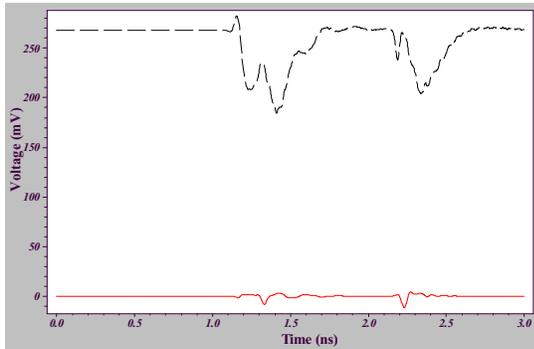
Figure 17: Dotted graph represents the difference between the signals on points OP1 and OP2 of the differential receiver in Figure 15. This represents the input noise signal to the differential receiver (peak input noise is 83mV). The solid graph represents the output of the differential receiver, OP3, in Figure 15. (peak output noise is only 4mV).
