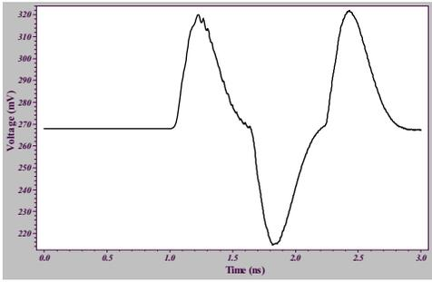
Figure 12: The difference between the signals on points OP1 and OP2 of the differential in Figure 10. This represents the input noise signal to the differential receiver (maximum cross-talk noise is only 53mv).
