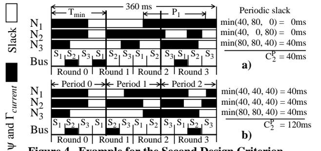
Figure 4. Example for the Second Design Criterion
