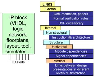
Figure 6. An IP block and its associated set of hyperlinks to hypermedia artifacts.
