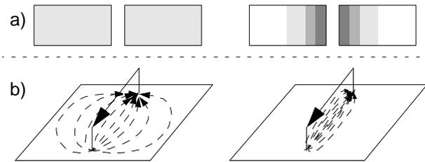
**Fig. 13:** a) Current distribution for signal line and its return; b) Current flow for a signal line over a ground plane; Left is low frequency, right is high frequency for both.
