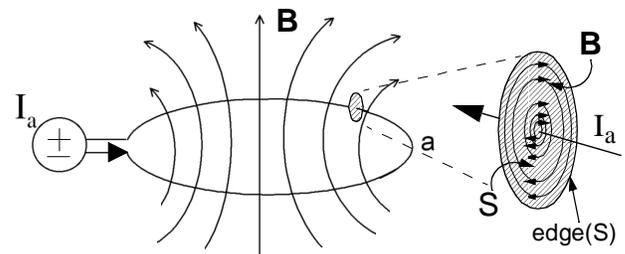
**Fig. 1:** Magnetic Field created by a time-variant current flowing through a conductor loop.
