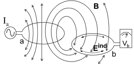
**Fig. 3:** Magnetic field created by the time-variant current in loop **a** induces voltage in a second loop, **b**, since some of the magnetic field passes through **b**.
