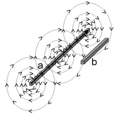
**Fig. 10:** Ampere's Law: Current flowing through segment **a** creates magnetic field.
