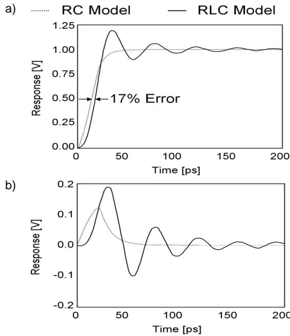
**Fig. 6:** Results for 32 bit bus structure in Fig. 5. *a)* shows the voltage response at the far end node of the active line, while *b)* shows the response at the far end node of the immediately neighboring ‘quiet’ line. The input was a 20 ps ramp from 0–1 volt.
