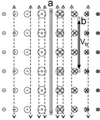
**Fig. 11:** Faraday's Law: Time-variant magnetic fields (circles and crosses indicate direction) create induced electric fields (dashed lines) which in turn create voltages in victim line **b**.
