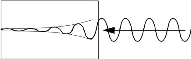
**Fig. 14:** Attenuation of electromagnetic wave as it passes through a conducting material.
