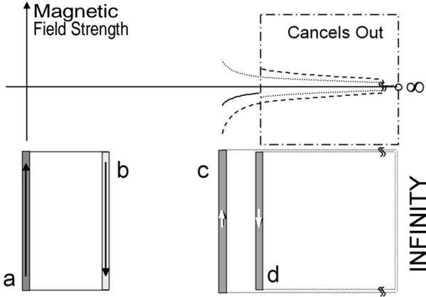
**Fig. 9:** Loop inductances reconstructed from partial couplings. **a** and **b** carry current, **c** and **d** have the shown orientation. The plot shows the magnetic field of **a**'s current (dotted) and **b**'s current (dashed) over the virtual loops of victim segments. Where the loops of **c** and **d** overlap, the flux from **a** and **b** cancels and what is left (solid line) is *exactly* the loop coupling similar to Fig. 3.
