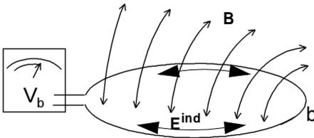
**Fig. 2:** Electric voltage created by time-variant magnetic field passing through a conductor loop. The integral of the magnetic field over the loop area is referred to as the *magnetic flux*.
