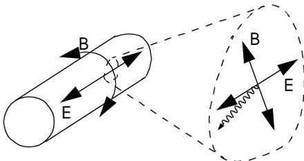
**Fig. 15:** High frequency electric/magnetic field form electromagnetic wave penetrating the surface of a cylindric conductor.
