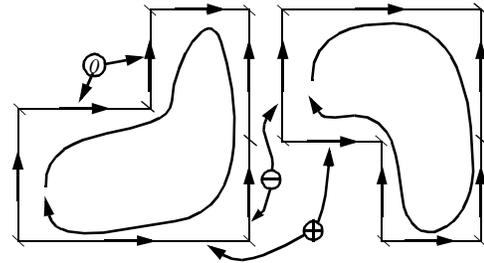
**Fig. 8:** Representation of current loops through partial inductance elements. The short arrows show the current directions, the long arrows identify the loop interactions. The signs of the  $S_{ij}$  terms are shown for selected segment pairs.
