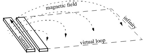
**Fig. 7:** Loop definition of partial inductance.
