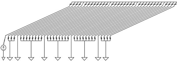
**Fig. 5:** 32 bit bus with four in-plane return lines. Leftmost line is active. Line numbering from left to right.
