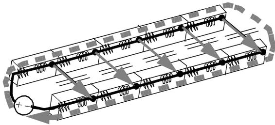
**Fig. 12:** Current return paths for loop inductance calculation. With capacitance (solid thick lines) and ignoring capacitance (dashed thick line). Mutual inductances not shown in this figure.
