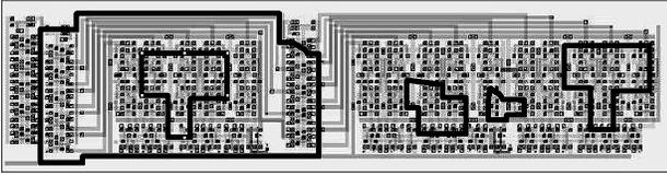
**Fig. 4:** A sample circuit with a few possible conductor loops formed by the interconnect wires.
