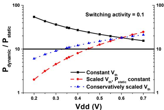
Figure 4. The ratio of dynamic to static power drops when using low  $V_{th}$ 's to reduce delay penalty in low  $V_{dd}$  gates. 35-nm technology is modeled.
