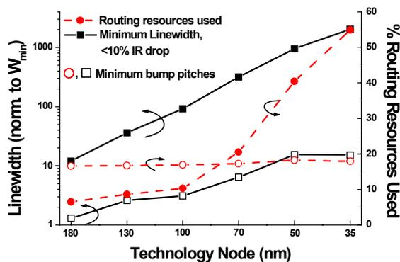
Figure 5. IR drop scaling trends based on minimum allowable bump pitch (open symbols) and ITRS bump/pad count projections (solid symbols).
