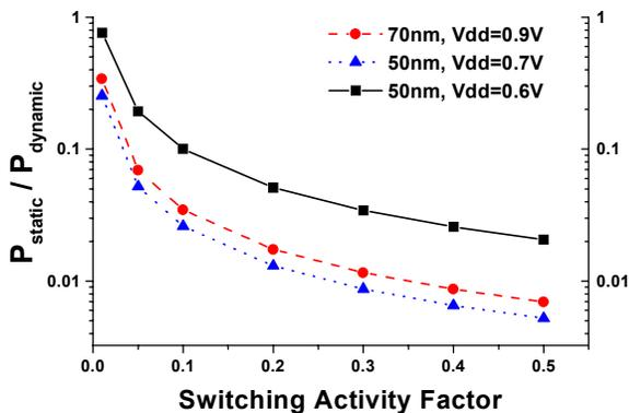
Figure 1. The ratio of static power consumption to dynamic power for an inverter with fan-out of 4 and average wiring load. Temperature is 85°C.
