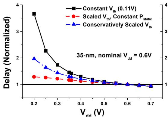
Figure 3. Delay increase due to  $V_{dd}$  reduction can be effectively offset by reducing  $V_{th}$ .
