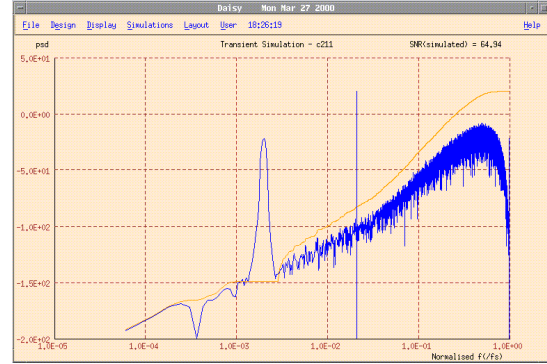
Fig. 4. The power spectral density plot for a finite OTA gain of 3000 and a finite OTA GBW of 50 MHz.
