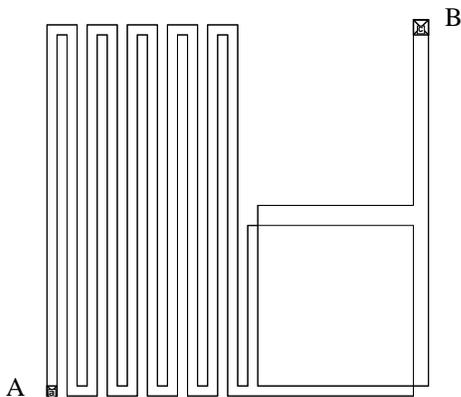
Figure 3: Layout of a poly resistor (grey) on top of which a metal plate capacitor (black).
