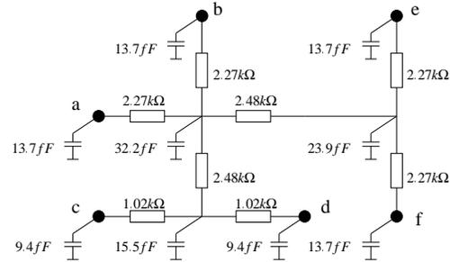
Figure 8: Circuit extracted from layout of 6-terminal line with  $f_s = 5$  GHz
