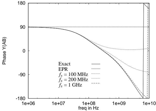
Figure 6: Phase of the trans-admittance of the RC structure.
