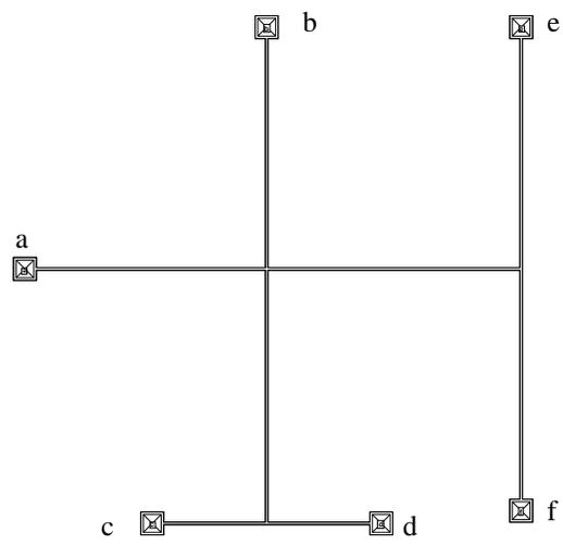
Figure 7: Layout of a 6-terminal poly line.
