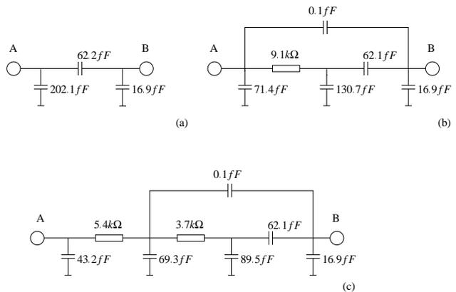
Figure 4: Circuits extracted from layout of RC network: (a) EPR model (b)  $f_s = 100$  MHz (c)  $f_s = 200$  MHz
