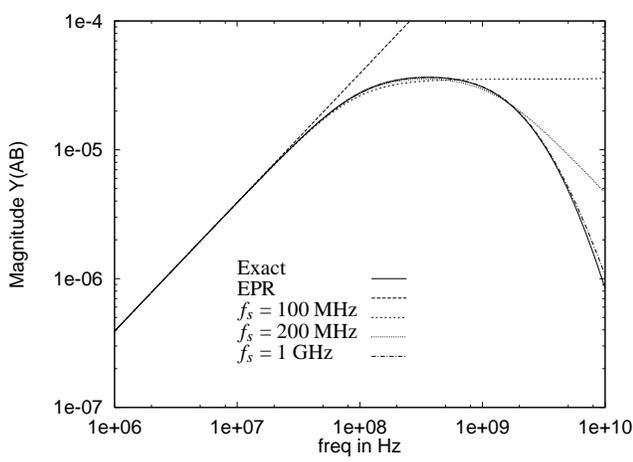
Figure 5: Magnitude of the trans-admittance of the RC structure.
