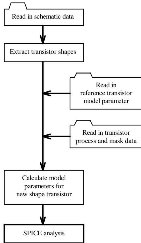
Fig. 10 Flow diagram for transistor model parameter generation program for various transistor shapes
