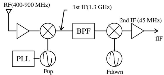
Fig. 2. Block diagram of double-super tuner
