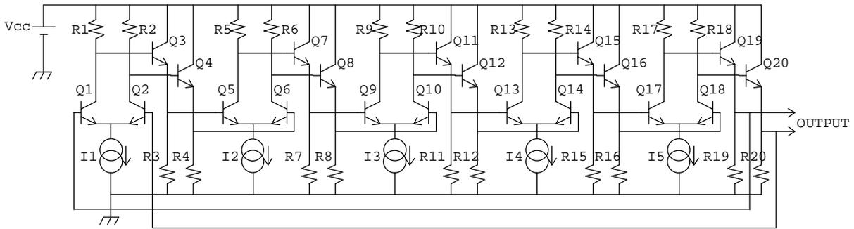
Fig. 11 Five stage ring oscillator
