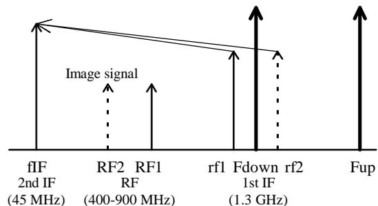
Fig. 3 Frequency spectrum of double-super tuner
