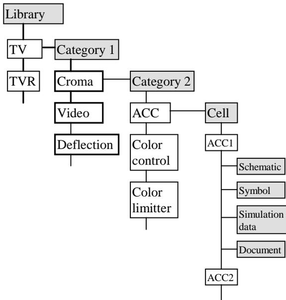
Fig. 6 Structure of an analog cell database
