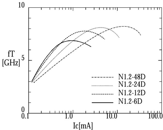
Fig.9 Transition frequency vs collector current for npn transistors.
