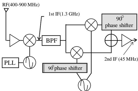
Fig 4. Block diagram of double-super tuner with image rejection mixer
