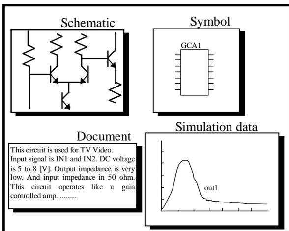
Fig.7 An example of an analog cell data
