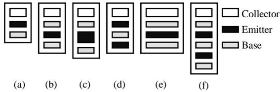
Fig. 8 Various transistor shapes in ICs
