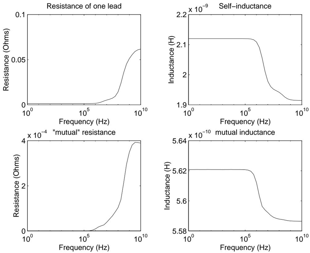
Figure 4: Inductance and Resistance of Package Leads as a Function of Frequency
