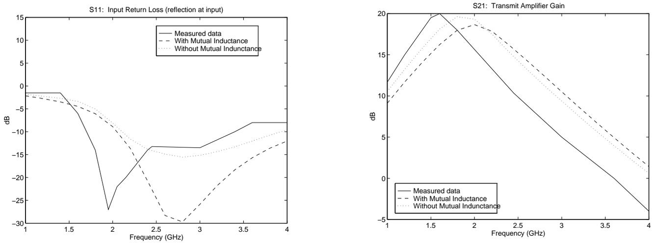
Figure 5: Simulation with Package and Bondwire Models, with and without Mutual Inductance
