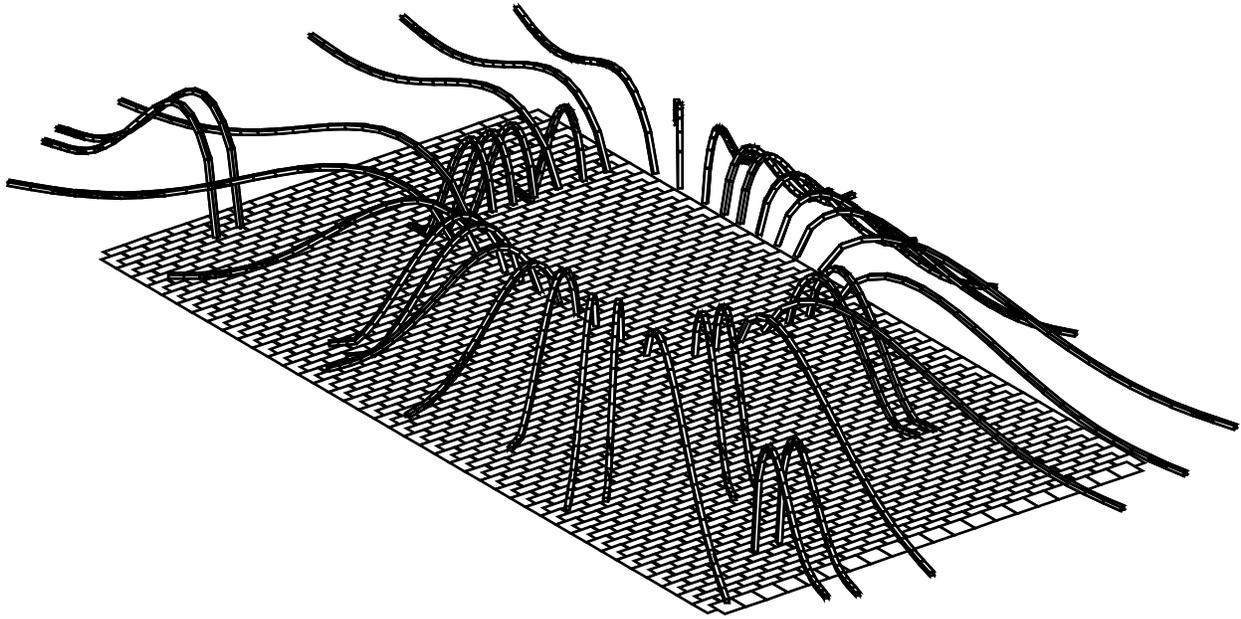
Figure 8: Bondwires with Ground Connections to the DA Plane
