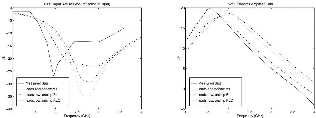
Figure 7: Simulation with Package, Bondwire, and On-chip Interconnect Models
