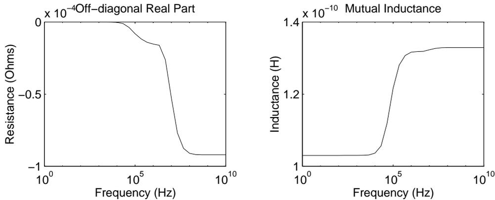
Figure 9: Mutual Inductance and Resistance Between Two Bondwires in Presence of Die Attach Plane
