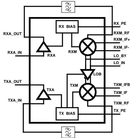
Figure 1: HFA3624 RF/IF Converter Block Diagram
