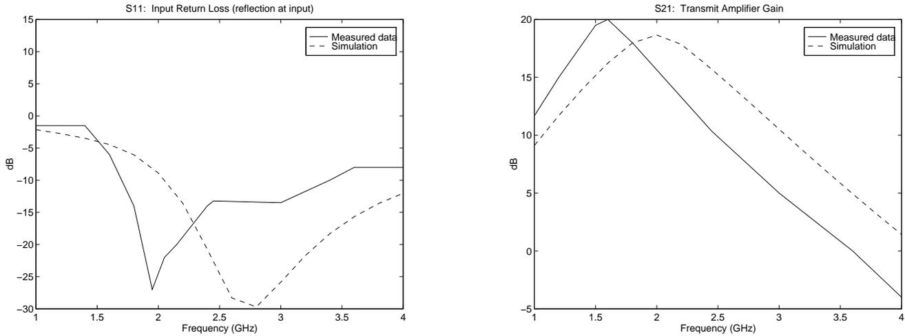
Figure 3: Simulation with Package and Bondwire Models
