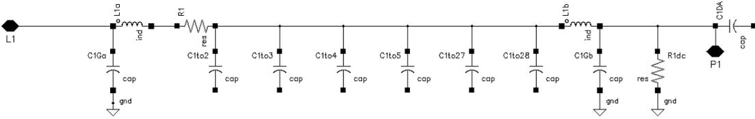
Figure 2: Lumped Element Model of a Single Package Lead
