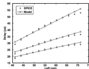
Fig. 3. Mean delay as a function of gate length for a NAND gate
