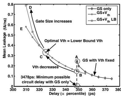
Fig. 5. Advantage of doing joint  $V_{th}$  and Gate Sizing
