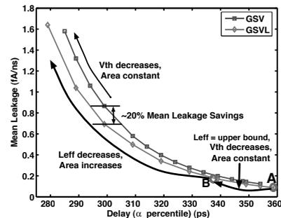
Fig. 6. Leakage-Delay tradeoffs for GSV and GSVL
